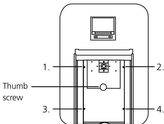
Unscrew the thumb screw to undo the passive accessory. Lift out the passive accessory. To fit an active accessory unscrew screws 1 to 4 and lift out the metal base plate.
