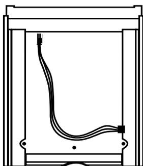
This will expose the bottom of the sample chamber with the power supply connection needed to operate the active accessories.
