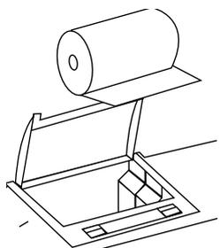
Insert the paper roll into the printer – ensuring that there is some paper sticking out of the printer before clicking the grey plastic back into place. Switch the instrument on. The power and error lights on the printer will flash. Once the instrument power on tests are complete press the feed button to check that the paper is fed correctly.
