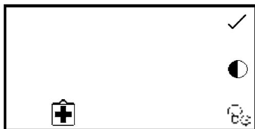
The lamp save function enables the time in minutes to be set after which the lamp will be turned off following a period of no lamp activity, i.e. no readings have been performed. This function is accessed through the instrument settings menu by pressing the key adjacent to the **lamp save** icon.
