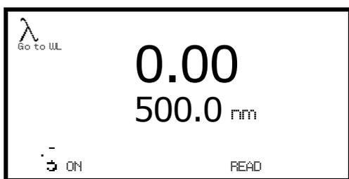
The **diagnostic** function allows simple checks to be carried out on the instrument. The wavelength can be changed, the lamp can be turned on and off and a sensitivity reading can be performed.
