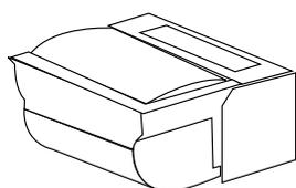
Unpack the printer from the packaging. Turn the printer upside down and connect the printer wires by clipping into the connector on the printer.
