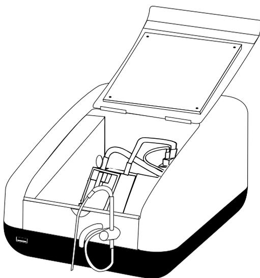
When the sipper accessory has been fitted and the tubing has been connected the instrument will look like this.
