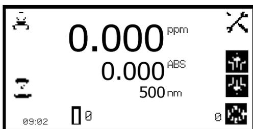
Press the key below the **8 cell turret** icon to highlight the icon and the two arrow icons above. Press the keys adjacent to the **arrow** icons to increase or decrease the current cell position of the turret, until the required sample position has been selected. Press the key below the **measure sample** icon. The instrument will perform a reading and display the result on the screen.
