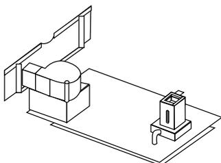
Take the peltier base plate. Connect the power supply in the bottom of the sample chamber to the connector on the underside of the base plate. Place the base plate in the sample chamber. Replace screws 1 to 4. Take the peltier front panel and slot into place before retightening screws 5 and 6.
