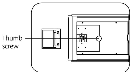
Unscrew the thumb screw to undo the passive accessory. Lift out the passive accessory. To fit a different passive accessory simply place the accessory in the correct orientation, align the thumb screw and tighten to fix in place.
