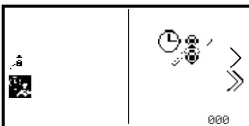
This stage allows an air gap to be added to the calibration sequence. If an air gap is not required press the key below the **000** icon to set the air gap to zero. If a previously programmed air gap is to be used press the key adjacent to the **double greater than** icon to skip this stage and retain the current air gap time.
