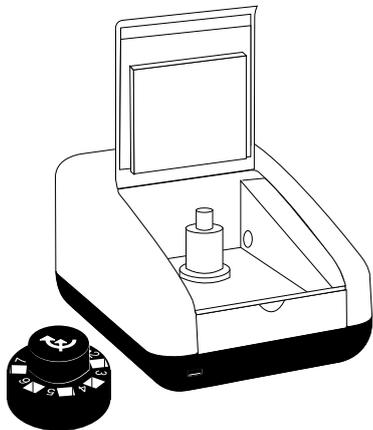
Take the 8 cell carousel and place on top of the motor, taking care to align the three ball bearings with the grooves on the motor shaft. Gently push the carousel down onto the motor shaft until it is located into place. Gently rotate the carousel until there is some resistance. The carousel is now in the correct position.
