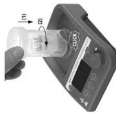
Fit the tube carefully and ensure it is properly attached.
