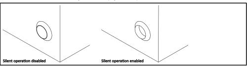
Activating silent operation on the temperature control unit reduces the noise level by decreasing the pumping capacity. For the exact position of the button **>Change pump speed< [114]** please refer to the "Wiring diagram" from page 68 in Section **»Annex«**.
