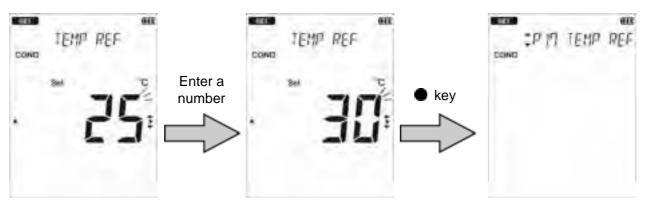
To return to the measurement mode, press the 🔊 key.
