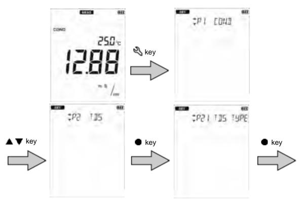
4. Press the **I** keys to select the TDS method and then press the **I** key.
