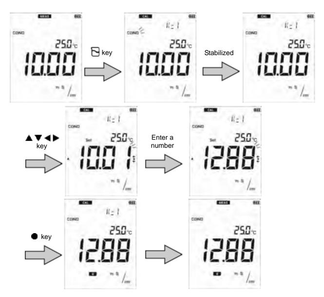
For multiple point calibration, repeat the steps 1. to 5. The calibration points are up to 5 points.
