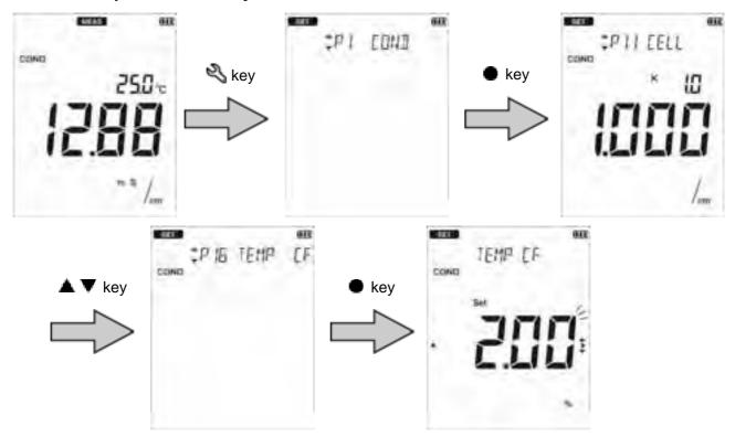
Press the ▲ ▼ ◀ ► keys to enter the temperature coefficient and then press the ● key to confirm.
