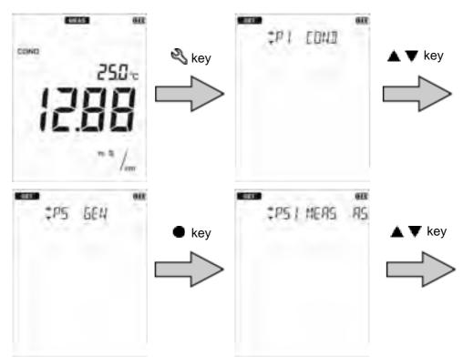
3. Press the ▲ ▼ keys to select "AUTO OFF" (automatic power off setting) and then press the ● key.
