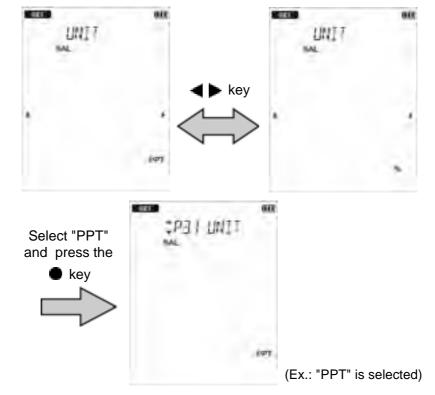
4. Press the  $\triangleleft$  keys to select the unit and press the  $\bullet$  key to confirm.
