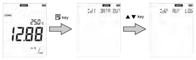
Enter the interval of saving in seconds and press the ● key. An interval from 0, 2 s to 3600 s can be set. When "0" is entered, this function is set to OFF. 4. Enter the period of saving in minutes and press the key.
