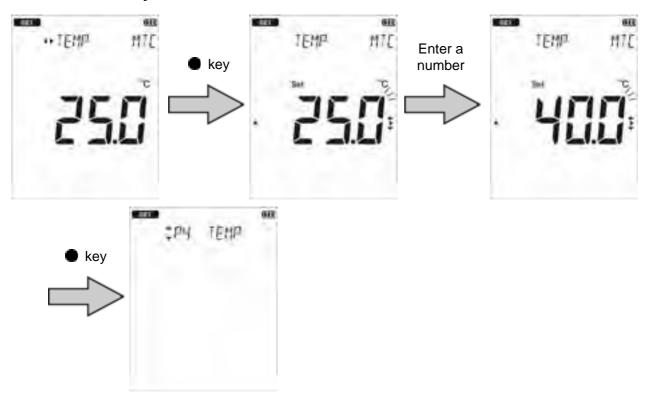
3. In the case of "MTC", enter the temperature to be compensated for and press the • key to confirm.
