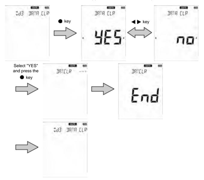
To return to the measurement mode, press the  $\infty$  key.
