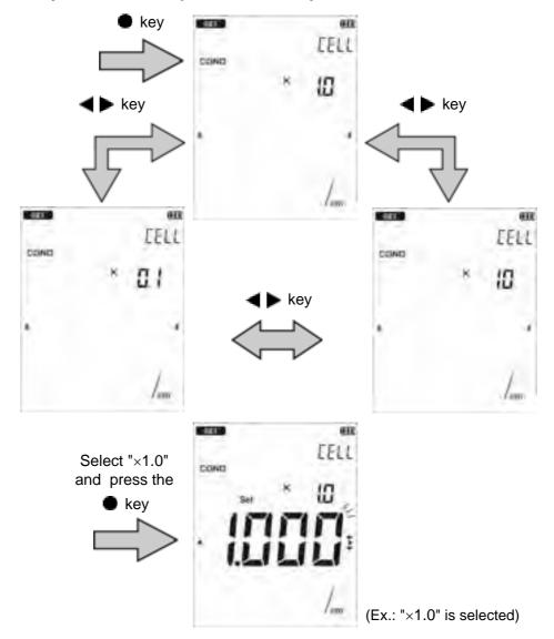
4. Press the ◀ ► keys to select the digit number of the cell constant of the conductivity cell and then press the ● key.
