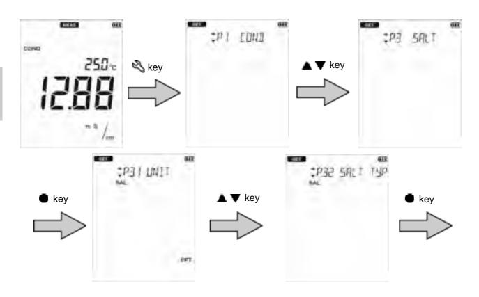
4. Press the <i>keys to select the salinity calculation method and then press the
