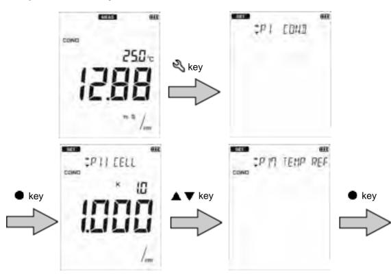
4. Press the ▲ ▼ ◀ ► keys to enter the reference temperature and then press the
