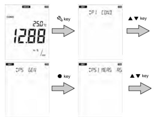
3. Press the  $\blacktriangle$   $\bigtriangledown$  keys to select "RESET" (initialize) and then press the  $\bigcirc$  key.
