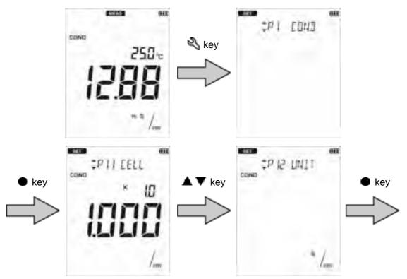
4. Press the **I** keys to select the unit and press the **I** key to confirm.
