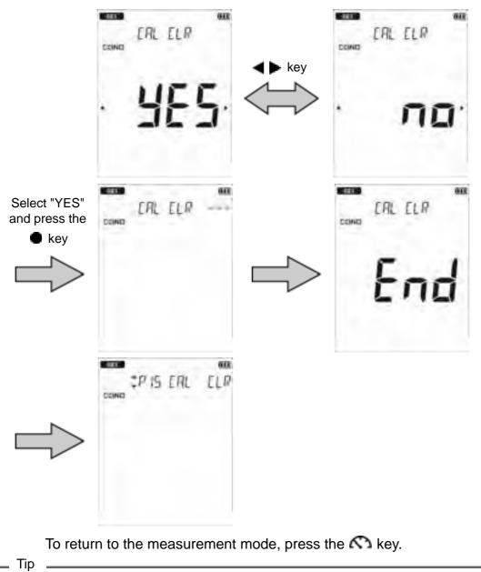
When the Seconds in the measurement mode, "CALCLR" screen appears, and the calibration data can be deleted.
