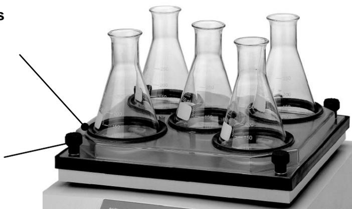
located in the four corners. Load Erlenmeyer flasks in cut-outs. To ease loading, slightly tip flasks. For proper seating, the cut-outs feature a preformed packing.
