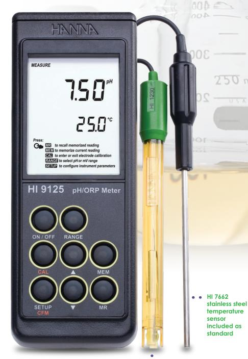
HI 1230B double junction pH electrode minimises junction contamination and enhances accuracy (supplied as standard)
