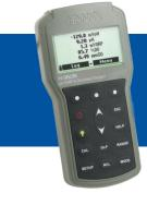
HI-98196 can transfer data to a computer via a USB connection and Windows® compatible software (not included)
