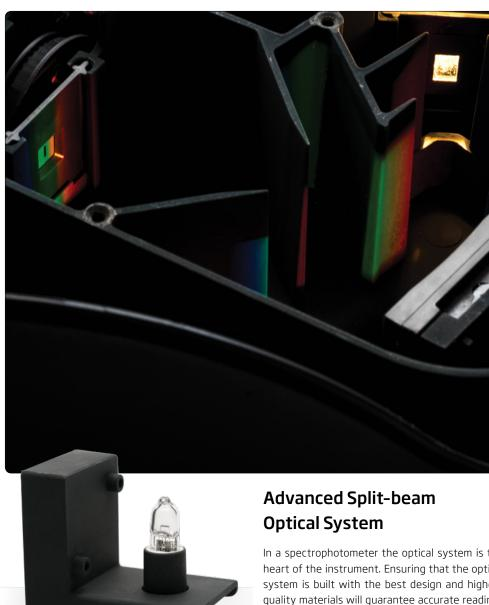
In a spectrophotometer the optical system is the heart of the instrument. Ensuring that the optical system is built with the best design and highest quality materials will guarantee accurate readings and a long life for the meter. When developing this meter our research and development team payed special attention to details and combined many small improvements to a typical spectrophotometer design to create a portable meter with unprecedented performance.
