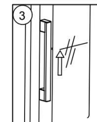
c. Raise the handle after securing the handle and holder.
