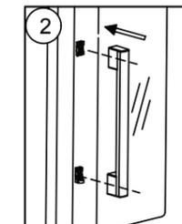
b. Align the handle with the holder on the door.
