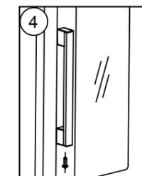
d. Use screws to fasten the handle at the bottom.
