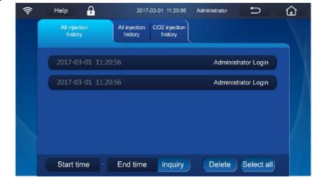
Enter/input "Start time-End time", and then click "Inquiry" to query the spraying record in this interval.
