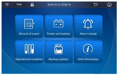
• **Record of event:** It can be used to query the records of door opening/closing, setting & modification, data upload/ download and account login.
