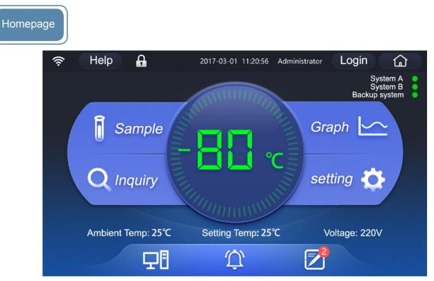
In the home page, it can display the real-time internal temperature, ambient temperature, set temperature, input voltage, backup system state (optional), network state, electromagnetic lock state (optional), user login status, freezer health status, temperature curve, and message/ note book, etc..
