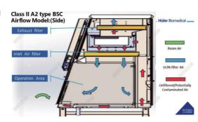
The biosafety cabinet is a negative pressure filtration and exhaust cabinet used to prevent the operator from being exposed to the bio-aerosol generated during the experiment, ultimately to ensure the protection for the operators, the samples and the environment.
