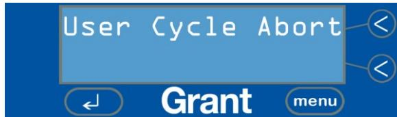
If the Level sensor is set to ON, and the fluid drops below the required level during operation, the cleaning cycle will stop and the following screen will be displayed.
