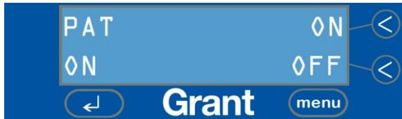
When the ON button is pressed, both the heater and the ultrasonic generator will turn on, irrespective of any other programmed settings.
