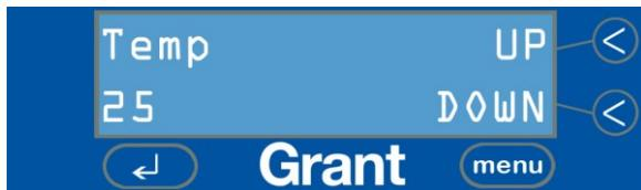
Use the UP and DOWN keys to accurately set the desired temperature of the cleaning fluid between ambient+5°C and 70°C.
