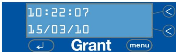
To change the time and date, scroll through the settings by pressing the MENU key and amend by pressing the UP and DOWN keys. When all the settings are correct, press the MENU key to move to the next screen.
