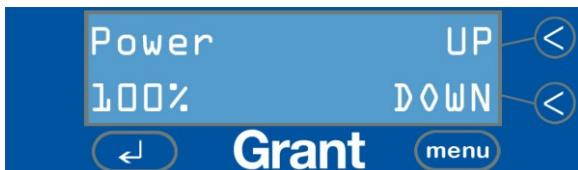
Use the UP and DOWN keys to scroll through the numbers between 50 and 100%. When the desired power level has been selected, use the MENU key to move to the next screen.
