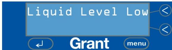
The Grant digital ultrasonic bath will not operate again until the tank is filled to the correct level.
