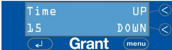
When the desired cycle time has been selected, use the MENU key to move to the next screen. This time setting will be saved until changed again in the Operator menu.
