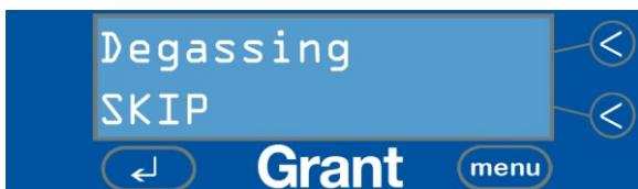
When you are satisfied that the liquid is degassed; i.e. when you can no longer see these bubbles forming and rising to the surface, press the ← key.
