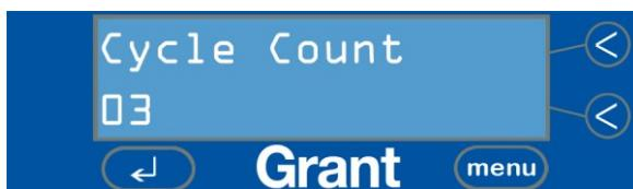
The cycle count shows all cycles which the bath has begun and includes those cycles which are not completed; i.e. those cycles aborted by the operator or because the fluid level was low.
