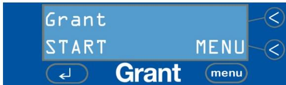
To scroll through the menu, press the MENU key. To exit the MENU at any time, press the  $\leftarrow$  key.
