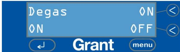
Use the ON and OFF keys to select the required option. (See page 23 for the importance of degassing.)
