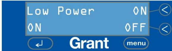
Setting Low Power to ON means that after five minutes of inactivity, the Grant digital ultrasonic bath will enter its SLEEP mode – the screen illumination will power down, and the internal water heater will not operate.
