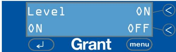
The level sensor is a resistive device, so will not detect fluids with very low conductivity such as pure deionised (DI) water.
