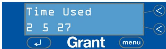
For example, the screen above shows that the bath has been in use for a total of 2 days, 5 hours and 27 minutes.
