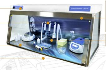
Built-in UV cleaner - recirculator both increases the maximum density of UV light and generates 25 m3/h air flow exchange prevents unwanted contamination and protects the user from direct UV light (in the upper hood) during manipulation
