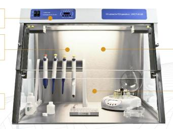
Built-in UV bactericidal cleanerrecirculator (patented) both increases the maximum density of UV light (in the upper hood) and generates 25 m<sup>3</sup>/h air flow exchange - prevents unwanted contamination and protects the user from direct UV light during manipulation
