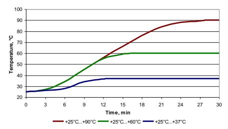
Fig. 6. Kinetics of liquid heating inside a single cell in a plate, total volume 1000 mcl
