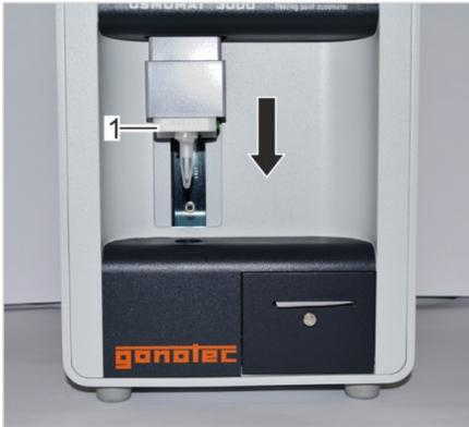
3. Move elevator (Fig. 129/1) down.
