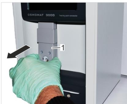
Fig. 98: Remove elevator cover
