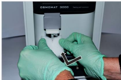
Fig. 20: Position transport safety device
