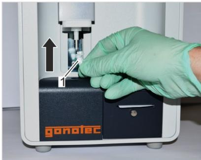
Fig. 19: Position measurement vessel
