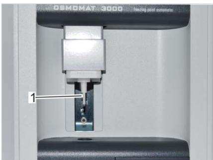
Fig. 46: Clean temperature sensor
