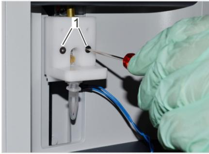
Fig. 100: Remove mounting screws
