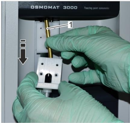
Fig. 101: Remove temperature sensor
