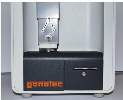
5. Remove the 2 mounting screws (Fig. 131/1) using Allen key (SW 2).
