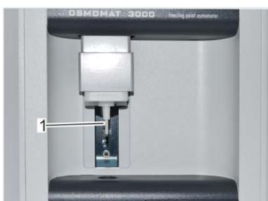
Fig. 57: Clean temperature sensor
