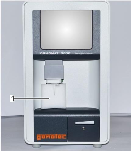
Fig. 24: Transport safety device
