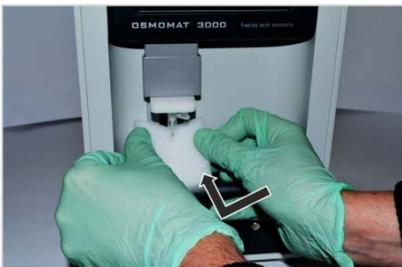
Fig. 149: Position transport safety device
