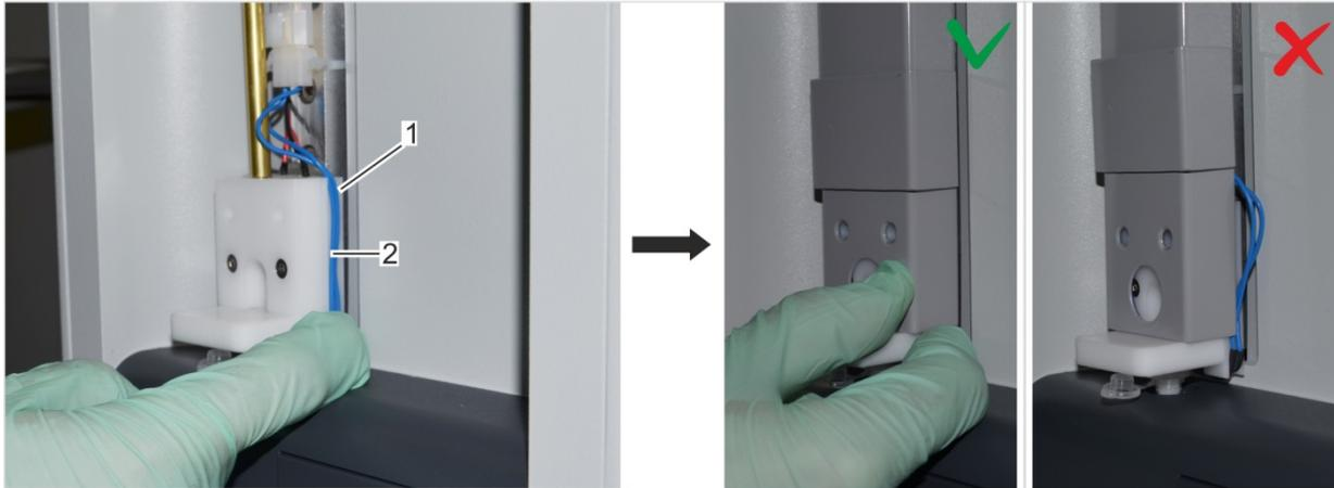
Fig. 108: Elevator cover with correct cable routing
