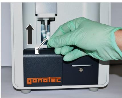
Fig. 128: Position measurement vessel
