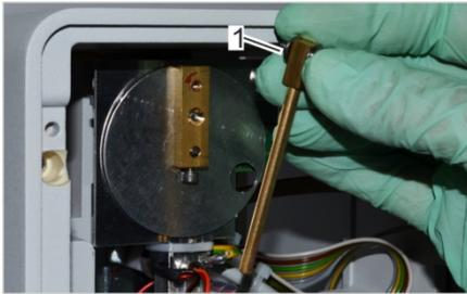
Fig. 87: Remove cryst-needle
