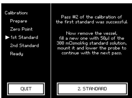
Fig. 77: Second calibration standard
