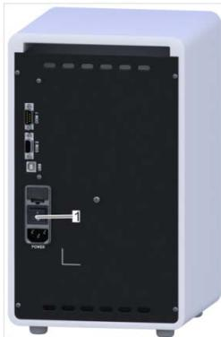
Fig. 81: Power down device
