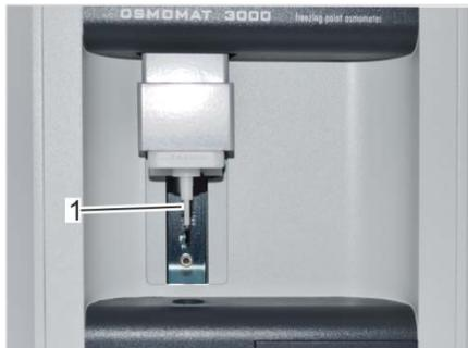
Fig. 56: Clean temperature sensor
