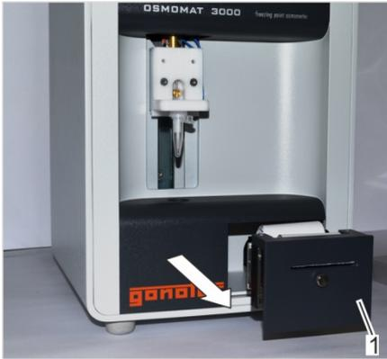
Fig. 117: Pull out printer
