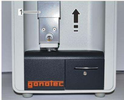
Fig. 96: Move elevator cover up
