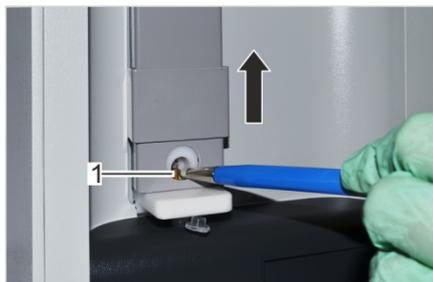
Fig. 110: Clean cooling nipple
