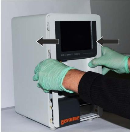
1. Install device front panel on device and push into place (Fig. 137).
