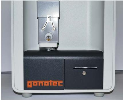
Fig. 139: Tighten mounting screws
