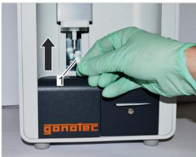
Fig. 146: Position measurement vessel
