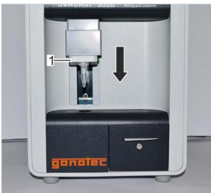
Fig. 54: Move elevator down
