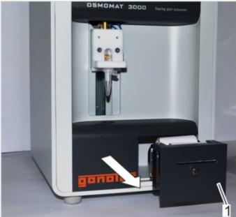
Fig. 26: Pull out printer
