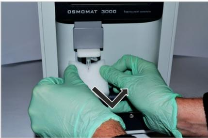
Fig. 25: Remove transport safety device
