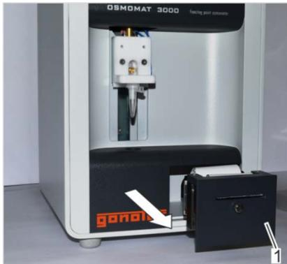
Fig. 133: Pull out printer
