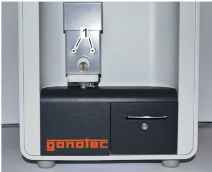
Fig. 109: Tighten mounting screws
