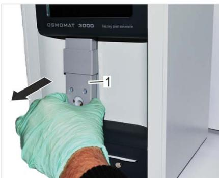
6. Remove complete elevator cover (Fig. 132/1).
