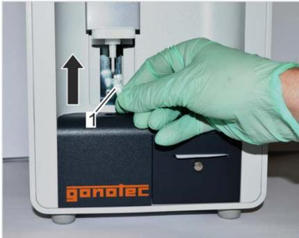
Fig. 52: Position measurement vessel
