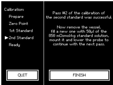
Fig. 78: Complete calibration
