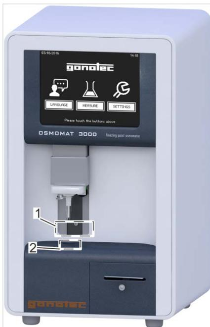
Fig. 142: Inspect device for foreign objects
