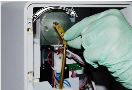
Fig. 92: Check free movement of cryst-needle
