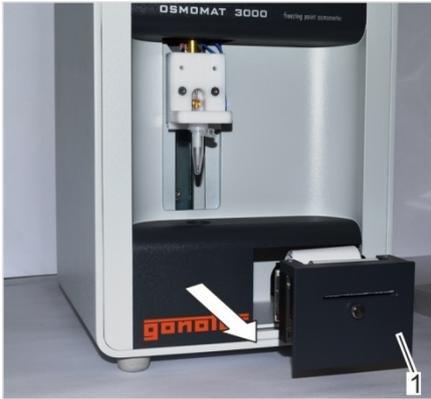
Fig. 123: Pull out printer
