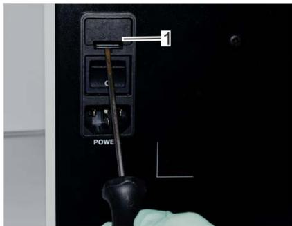
Fig. 112: Open microfuse cover
