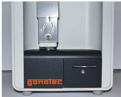
Fig. 97: Remove mounting screws
