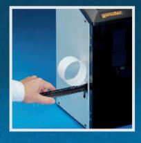
The measuring results are stored and are printed by order of the user You take out the sample holder after approx. 23 minutes and you can continue with the next serial measurements.
