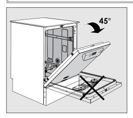
■ Open the door to an angle of approx. 45°. This ensures that the salt flows into the reservoir more easily.
