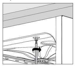
Screw the machine to the continuous worktop through the holes in the front trim on the left and right.
