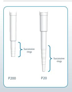
Successive rings have been positioned depending on the pipette volume range to guaranty the snug fit of tips throughout the protocols.
