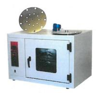
This dual purpose oven is designed to perform the loss on heat test and thin film test for bitumen and asphaltic materials and complies with the requirements of BS 2000 ASTMD6, D1754 & AASHTO T47, T179.
