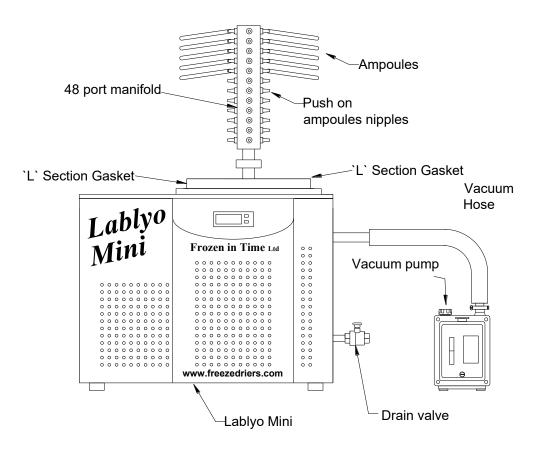
FIT/LYO/25/0 Lid with ampoule manifold 48-port
