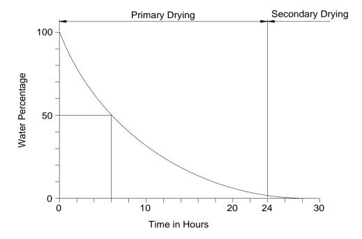
The drying time depends heavily on the vacuum level. The nearer the vacuum to the solidification point in accordance with the vapor pressure curve the shorter the drying time.
