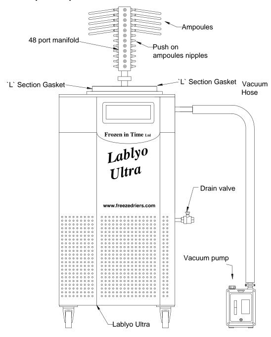
FIT/LYO/25/0 Lid with ampoule manifold 48-port
