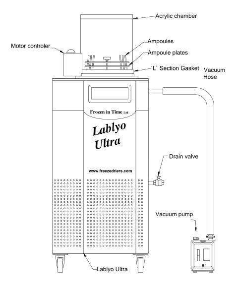
FIT/LYO/28/0 Spin Freeze with 1 x set carrier plates
