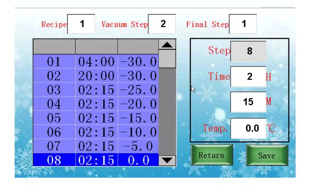
The program steps create a recipe to allow simple automation of the product chamber temperature using time to initiate the change in temperature.
