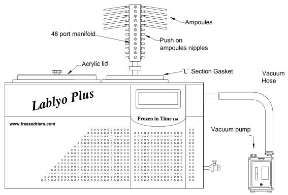
FIT/LYO/25/0Lid with ampoule manifold 48-portAdditionally requires:FIT/LYO/40/0
