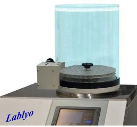
The long thin ampoules sit at an angle with the tops facing in slightly towards the centre. The vials are left to spin on an adjustable timer while the vacuum is applied. The centrifugal force will stop the product from overflowing and a long thin tapered layer will freeze up the side of the slanting ampoule maximizing the surface area.
