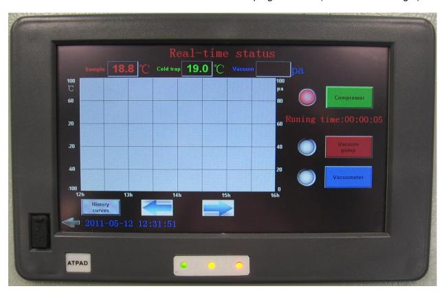
The main screens buttons are on the right, Compressor (green button), vacuum pump (red button) and Vacuum sensor (blue button)
