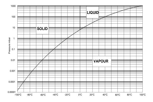
Fig. 3.1a Phase diagram for solid, liquid and vapour
