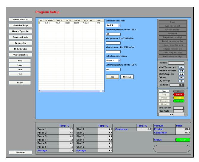
The Program setup screen is for programming the automatic freeze drying cycle. To change to another screen there are selection buttons down the left side as on previous pages.
