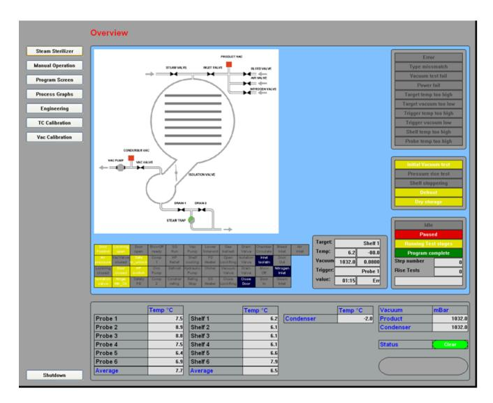
This screen is for is an overview of the freeze drier it shows what parts of the freeze drier are running.
