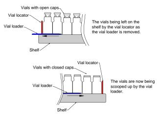
There are 6 usable shelves and each shelf holds 3 vial trays. The vial locators can hold various diameters of vials. Shelf spacers can be removed and replaced with the correct sized spacer to suit any vial height. Each of the shelves can be placed at differing heights in any combinations to suit.
