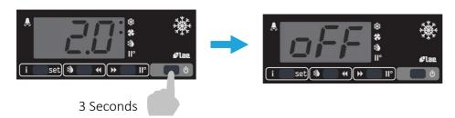
This will show while the unit is not operating but still has mains power applied to it. This mode may be used for interval cleaning regimes and short periods when the unit is not required. For extended periods of inactivity the mains supply should be isolated.
