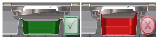
Do **NOT** block the fan airflow
