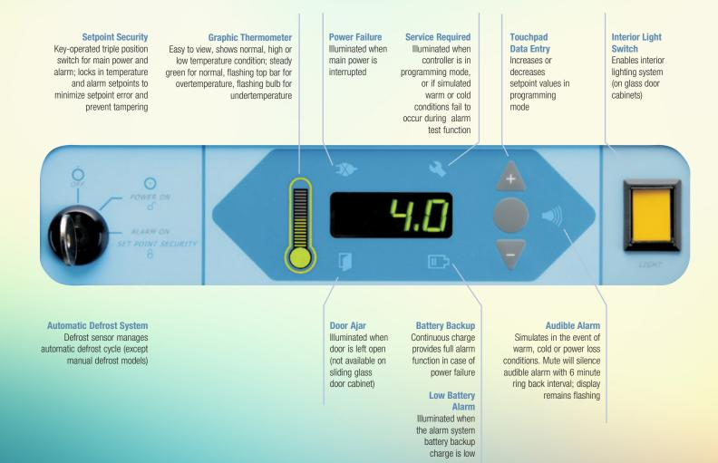
Our bright, easy to read display lets you know at-a-glance if your unit is running within range. Visual and audio alarms are designed to alert you in the event of a problem. Immediate access to high and low temperature parameters with the press of a button.
