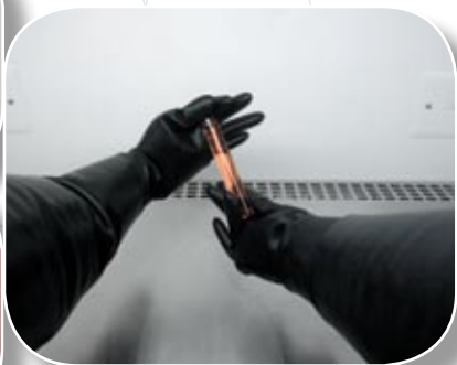
Neoprene™ synthetic arm-length gauntlets are flame and abrasion resistant. Single piece, leak-tested assembly guarantees maximum protection. Black color allows the detection of leaks by visual means.
