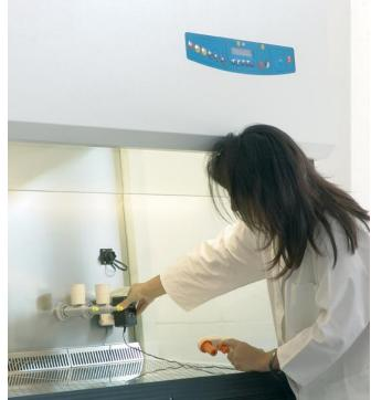
**Prefilters removal**: prefilters can be removed directly from the working chamber
