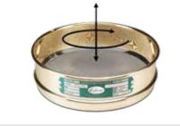
Vertical vibration is generated by the on/off frequency of the electromagnetic drive. However, vertical vibration is not enough to impart the correct movement for sieving. The shaker also needs to twist the sieve stack - this rotating action ensures the sample passes over the full surface of the sieve and the maximum number of apertures to give rapid accurate results
