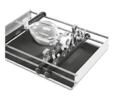
The cramp strips and spring strips are necessary for fastening separating funnels. The necks of the separating funnels are fastened in the grey plastic clamps, the spring strip secures the stoppers. The stems of the separating funnels are placed on a clamping strip h. For a modification of the standard rack system or in addition to the clamping strips h.
