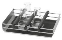
All flat-bottom vessels (Erlenmeyer flasks, beakers, test tube racks, sieves, etc.) can easily be fixed on the shaker with the clamping strips h. In addition to the clamping strips h supplied with the Combifix KS.
