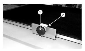
• Loosen the star-shaped knob (1) at the front of the shaking plate and move lever (2) to the desired position.
