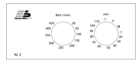
The operating panel for the listed shakers has two control knobs. With the left one the required speed can be adjusted (speed range see Technical Data!).
