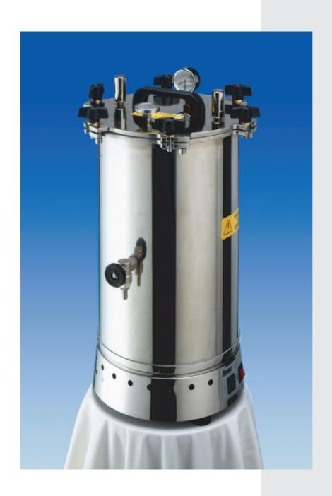
Compact and Fully Portable **Electronic Temperature Control** Simple and Safe Use **Domestic Electricity Supply** No Plumbing Needed Minimal Maintenance Required Electrically Safe To BS3456 Lid Locking Safety to H&SE PM73 Produced under ISO 9001 Suitable for Culture Media 121°C Operating Temperature 316 Stainless Steel Construction 22 Litre Capacity 280mm Internal Diameter 21.0Kg Net Weight
