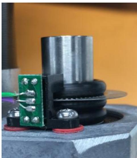
As shown in the figure, check if coded disc and the rubber ring on it are synchronously rotating with the shaft; if not, you should fix them with adhesive at the place where parts contact each other. Check whether the photosensor PCB is disordering. If it is, please replace the photosensor. Check the relative position of photosensor and coded disc. Coded disc should lie in the middle of photosensor notch, and coded disc cannot be contact with photosensor
