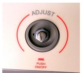
As shown in figure, take the knob, remove the screw and keep it well.
