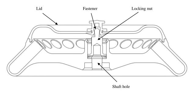
Figure 11-1 The rotor structure
