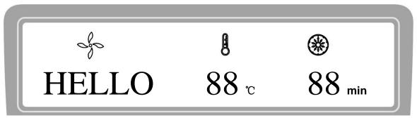
Figure 8-1 Self-checking interface
