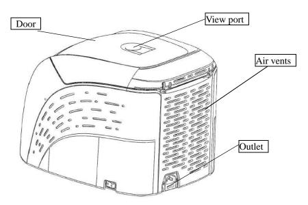
Figure 5.2 Rear view of the centrifuge
