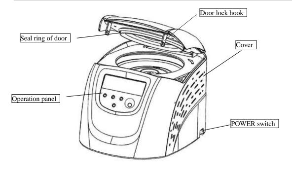
Figure 5.1 Front view of the centrifuge
