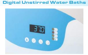
Digital water baths have push buttons for setting values. Temperatures can be easily and rapidly set with the push button, wipe clean control panel, featuring a bold LED display.
