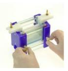
**4A)** Insert into casting base. Push the cams into the holes in the insert. Turn cams about 90° or until tight. Do not over tighten
