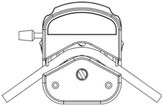
When installing the tubing make sure the tube follows its natural direction to avoid jamming and cracking of the tube. Moreover, straightened the tube to avoid tubing accumulation in the pump head.
