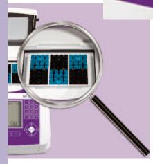
Intuitive user-friendly interface facilitates manual selection of different temperatures in each of the 4x4-well zones, for full user control during PCR optimisation.
