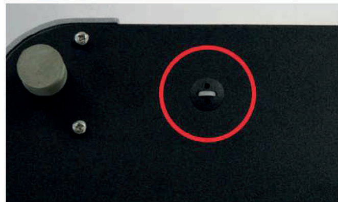
Mechanical Emergency Door Release on the downside
