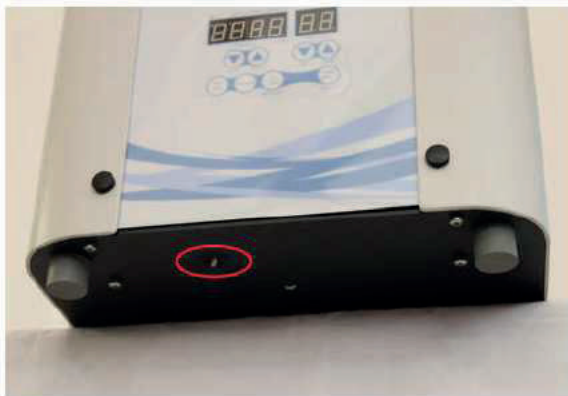
Over hang the machine to gain access to emergency lid release
