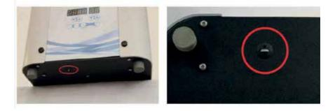
After replace the Plastic plugs back into their original position. Reconnect the centrifuge power line once the mains power has been restored. Check all is working correctly by closing the lid, wait 5 seconds then press lid open. If not working refit or Contact your Distributor
