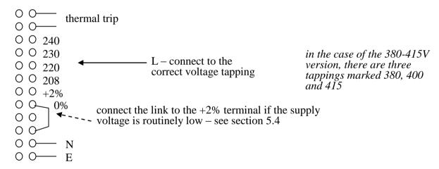
The thermal trip connection forms part of the circuit to the contactor coil.
