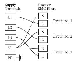
A model made to this diagram can be converted by the customer between the following supply voltages:
