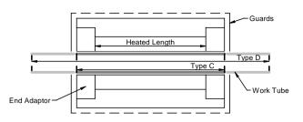
insulation. These may be blank (no hole) or may have a hole to suit a work tube, depending on the customer order. Additional adaptors may be ordered to suit different work tube sizes. Check that the end adaptors are correct for the tube: if not, seek advice from Carbolite. Small alterations to the hole in the adaptors may be made with a file, but first read the section on ceramic fibre safety (5.2).
