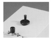
The Advance / Rewind control (on top of the microtome) is used to advance the specimen to the knife and for trimming. It is also used to reset the mechanism usually after cutting each specimen.
