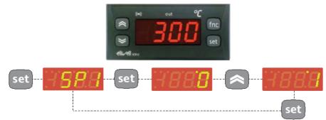
Once the 'SP1' label has been displayed, press the "set" button to display the Set point 1 value. The Set point value appears on the display. To change the Set point value, use the "UP" and "DOWN" buttons within 15 seconds.
