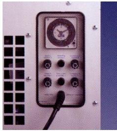
The segments of the clock are set in the factory such that day 1 is the first working day of the week (Monday). The rapid freezer is set to switch-ON at 08.00 hours and switch-OFF at 17.00 hours for days 1 to 5. The switch-off time is shown as Red on the Timer Segments. Please note the rapid freezer can take up to 60 minutes to reach its normal working temperature, so will be ready for use by 09.00 hours.
