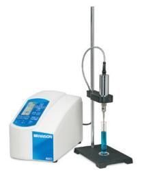
**Stand and Converter Holder:** The support stand with stainless steel rod accommodates Branson's 20 kHz converter. The converter holder supports the ultrasonic stack (converter and horn) and is easily adjusted to properly position the horn in the sample.
