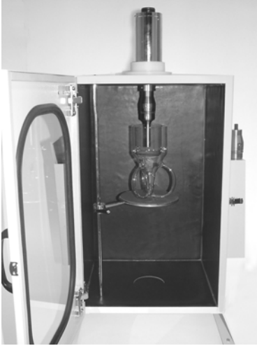
Figure 3.1 Converter/Horn Assembly in Stand. Set ON/OFF switch to OFF
