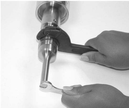
Figure 4.2 Connection or Removing Tip and Horn
