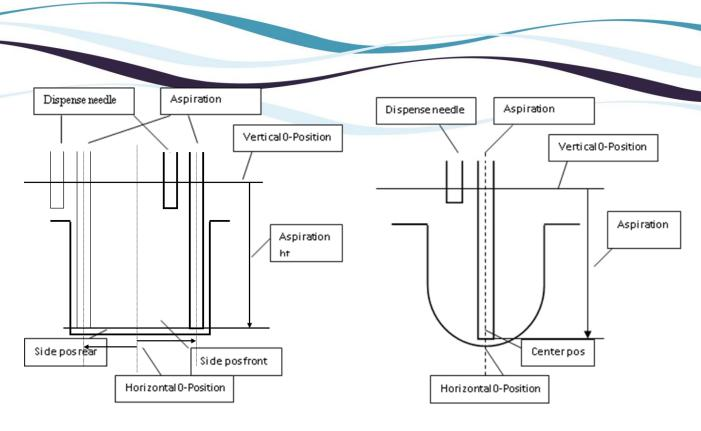
Drawing49.: Aspiration Positions for flat bottom or curved bottom plates
