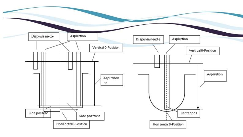
Drawing49.: Aspiration Positions for flat bottom or curved bottom plates
