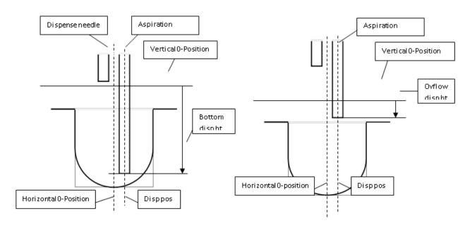
Drawing 50. Wash Positions for flat bottom and curved bottom plates
