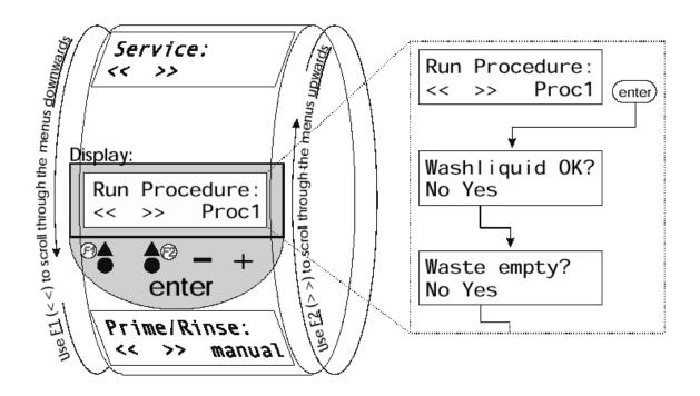
The software was designed to make navigation through the different menus as easy as possible. The main menus are organized like a wheel which can be turned in both directions by means of the two first keys (function key 1 <F1> and function key 2 <F2>). When pressing <F1> or <F2> the next respectively the previous menu will be displayed.
