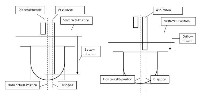
Drawing 50.Wash Positions for flat bottom and curved bottom plates
