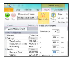
3. Individual multi-wavelength measurements are displayed in each well, with raw absorbance displayed on the right hand panel as a graph of absorbance vs. wavelength.
