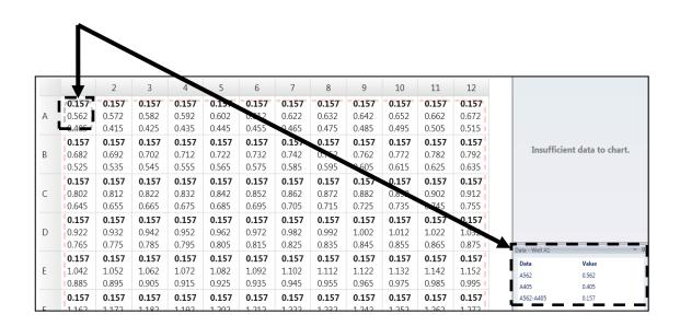
9. When users click onto a well, it is highlighted (dashed lines). In regards to dual wavelength measurements, three absorbance values are displayed.
