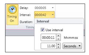
The measurement cycle (delay and interval) can be inputted and multiple cycles can be selected.
