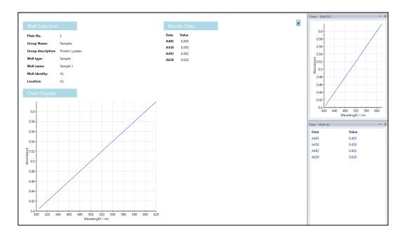
5. Results can saved to be 'Database'. A database is useful for saving, sharing and extracting data via communication with an external database system such as LIMS. Users can save files and templates onto database, 'File' (save to own personal file), or 'Save Method Template' (saves the method protocol for future use).
