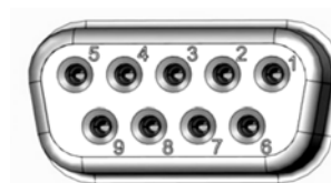
Figure 23: Sub D socket (9) “Object temperature input” in the VD rear control panel to connect the optional Pt 100 sensor
